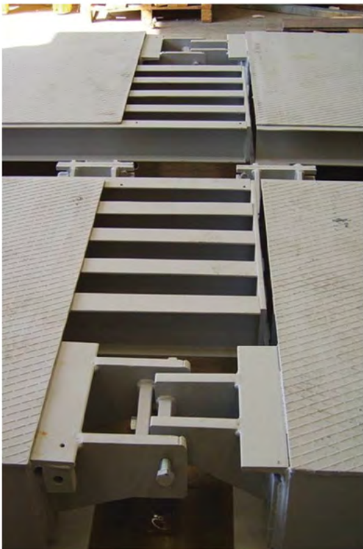
Load cell easy and direct access after top-plate removal
