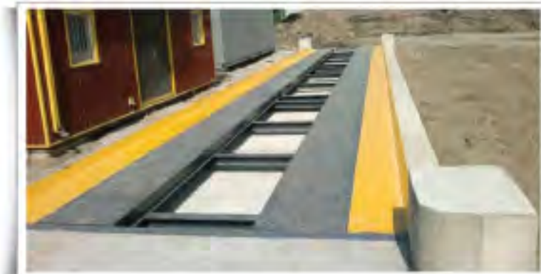
DIY-1000 Weighbridge. Gap in the middle
