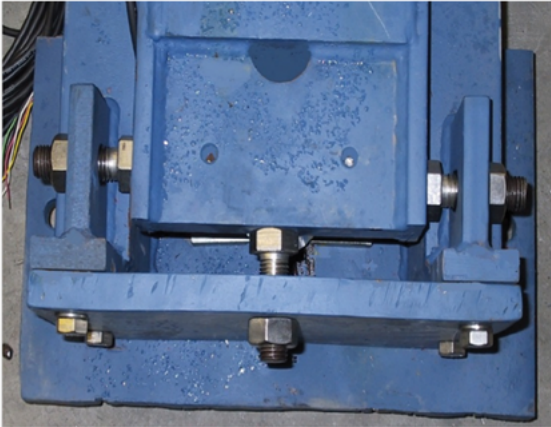
TS-300 weighbridge.2 direction buffering system
