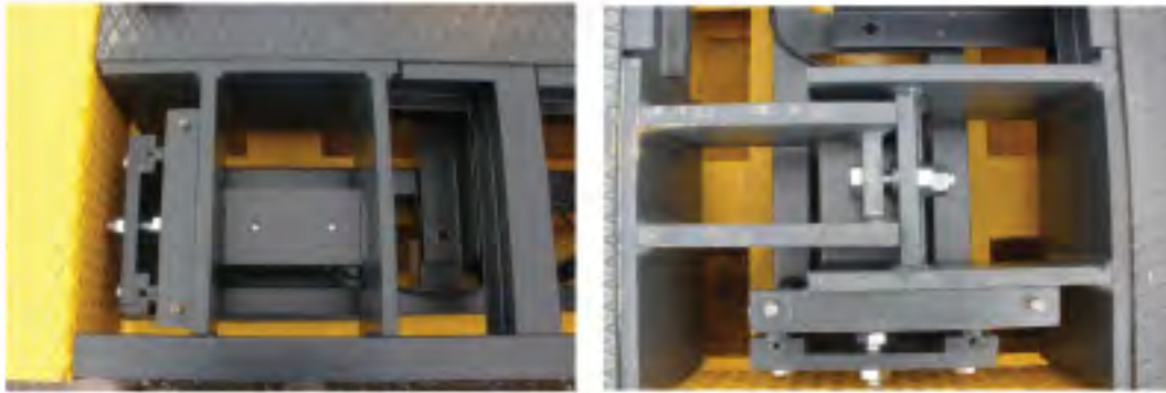
DIY Weighbridge support keys
